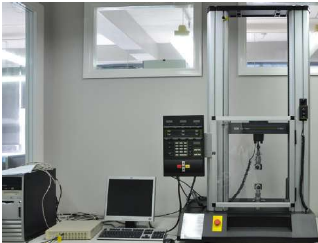
Fig. 2. Instron universal test machine – tear test set-up.
